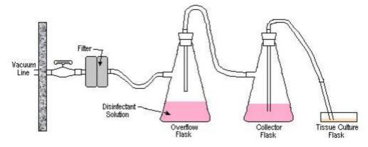
The above diagram depicts the proper set-up for vacuum lines that are used with potentially hazardous biological materials.
