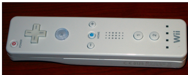
Fig. 1. The Wiimote has a large circular button, referred to as the A button. The three-axis accelerometer is in an area roughly beneath this button.
